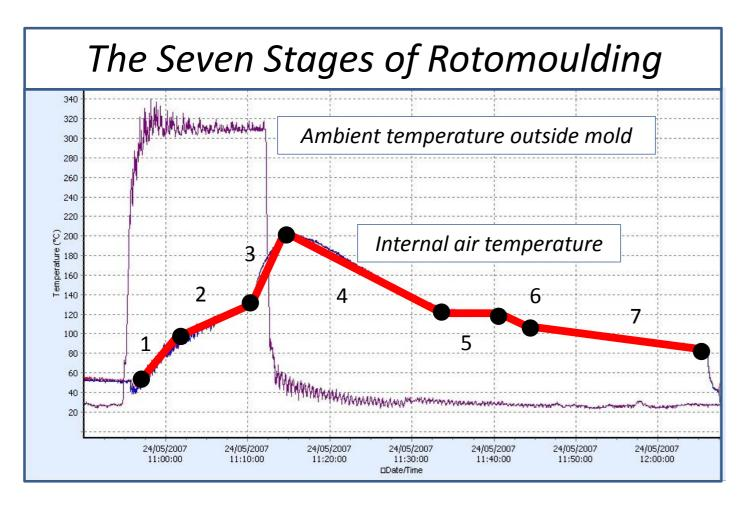
It helps to consider these events in a discrete fashion but this isn't the full picture and it doesn't happen like this in the mould. These events actually overlap each other in a very non-discrete way. For example melting does not just happen during phase 2 but instead it starts in phase 1. Consolidation does not take place in phase 3 but happens as soon as melting begins: phase 1. This is seen more clearly when we consider the temperature of the metal mould wall.
