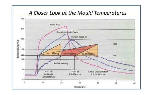
As soon as the mould wall temperature reaches the melting temperature of PE around 120C (248°F) the powder will begin to stick and melt. On a graph of the mould's internal air temperature you will see this starting to happen earlier than the beginning of phase 2! Similarly the cooling and subsequent solidification of the PE will begin to happen when the mould wall temperature drops below 120C (248°F), much earlier than the beginning of phase 5.
