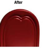
Then Persico prepared a CNC-milled aluminium mould for the production of the spoons. Finally, the actual 1.5-metre spoons were rotomoulded with Persico's moulds using regenerated polyethylene plastic. The 63 huge spoons positioned on the front of the hotel in a target motif – red ones encircled by white – are a sight to behold.
